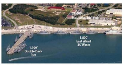
Capital-ship class 1,100-foot pier and the wharf area with its heavy load/unload capabilities.
